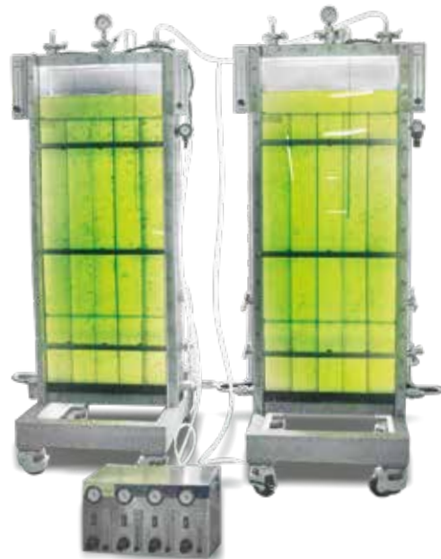
Pilot Scale, Plate Type Photo Bioreactor, Illuminated by Internal LED Plate
