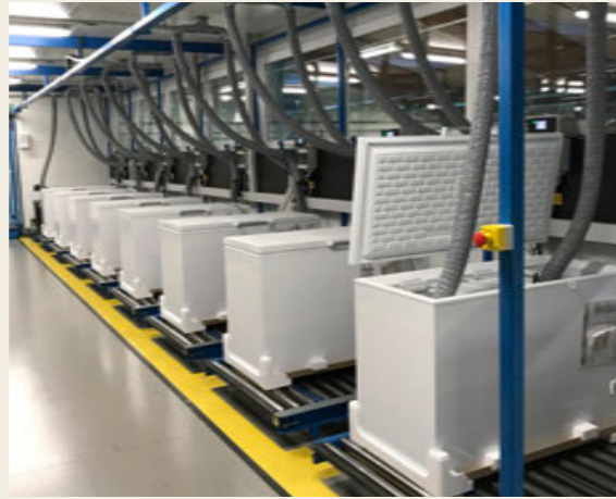
24h test being performed before shipment
