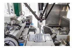
Every lens from our production line will have to pass through a high-definition inspection camera. The camera will detect imperfections such as cracks, scratches and any defects found on the lens. Defective lenses will be automatically rejected to ensure that only the best lenses are released to our consumers.
