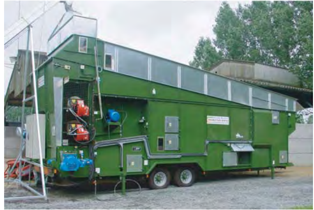
MDF 22000 Drier 25t/hr- full highway version
