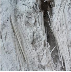
***Fibrotais** is a product which has yarns in fiberglass shape. It is used to reinforce plaster-renders, gypsum, cement mortars and concretes.*
