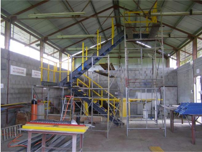
FRP structures designed and fabricated in-house being assembled for inspection by Clients.
