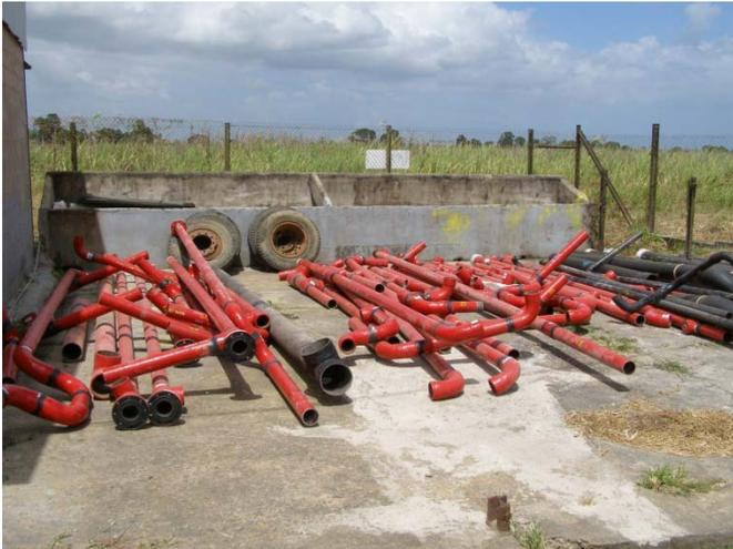
Conley Fire retardant pipe spools awaiting shipment to offshore platform. Pressure testing of each spool completed.
