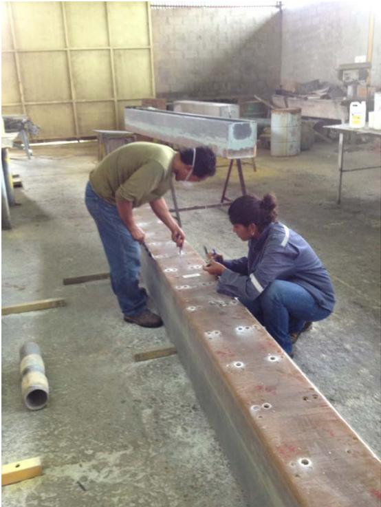
Flow distribution boxes for Petrotrin Acid Plant. Each box has 70 holes ranging 5/8" to 1-3/64" dia with 1/64" tolerance allowed.
