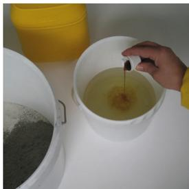
**Plais N** is a plasticizer for mortar and concrete, which is ideal to obtain an excellent plasticity, greatly facilitating their manageability and improving their work placement.
