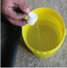
*Fiais* is a liquid additive in mineral base with high concentration that because of its exothermic reaction is able to decrease the freeze point of mix-water and increases the hydration of the cement allowing the concreting at low temperatures. (UNE-EN 934-2 and 3)
